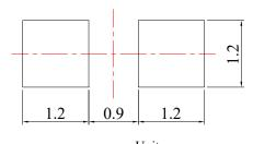
Unit: mm Tolerance: ± 0.10mm
